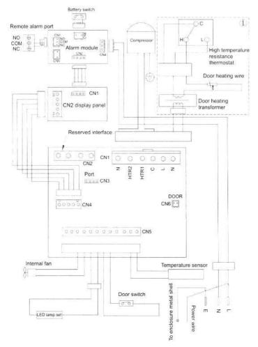
Note: The parts in the dashed box  $\ 1)$  are only applicable to HYC-118A series products.
