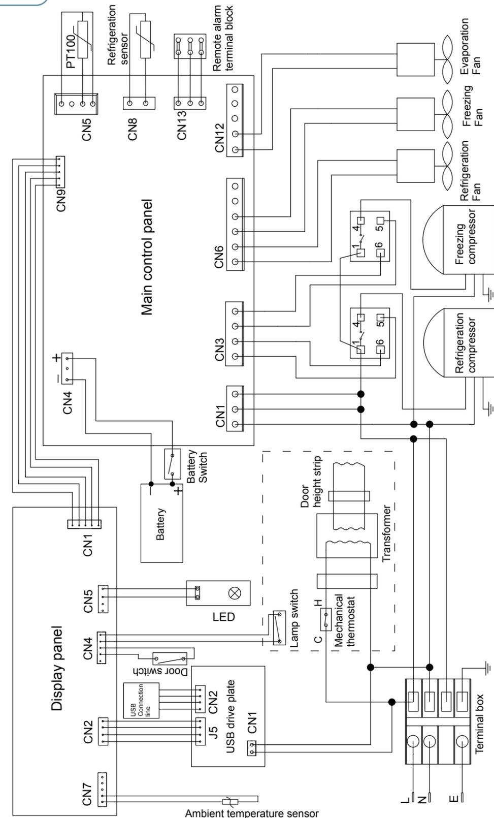
Note: The content in the frame with dotted lines are applicable for HYCD-282A series.
