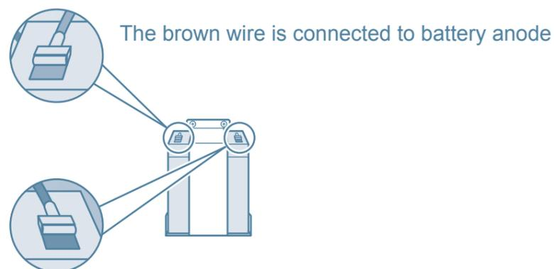
The brown wire is connected to battery anode
